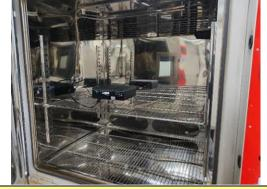
High Temperature and High Humidity Test/ Low Temperature Test
